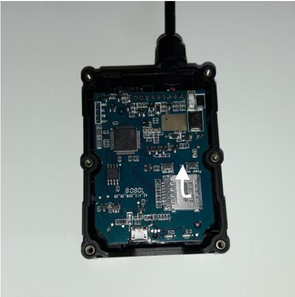
Locate the SIM card holder. Slide the metal plate LEFT to unlock and pull UP
