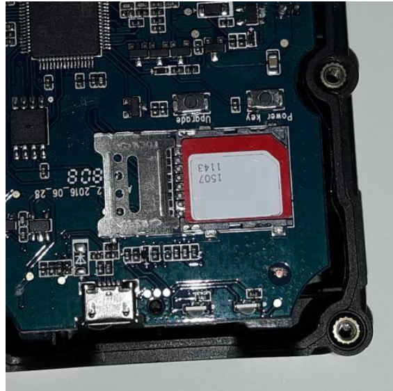
Position the Nano SIM in the slot, Flip close the SIM card holder metal plate, slide the metal plat right to lock.
